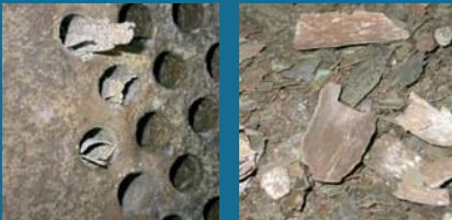
Tube bundle cleaning
