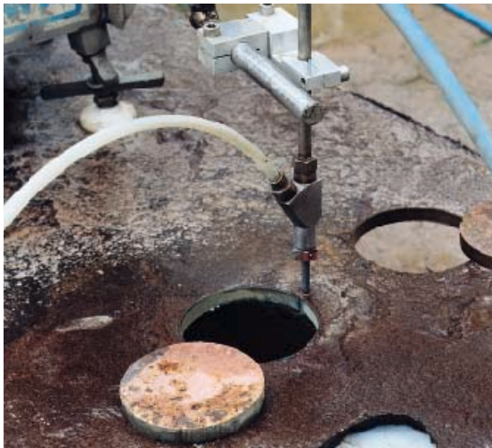
Cutting circular openings in steel plates
